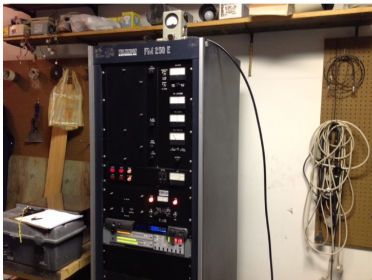
40 year old tube type FM transmitter at KIAM.
