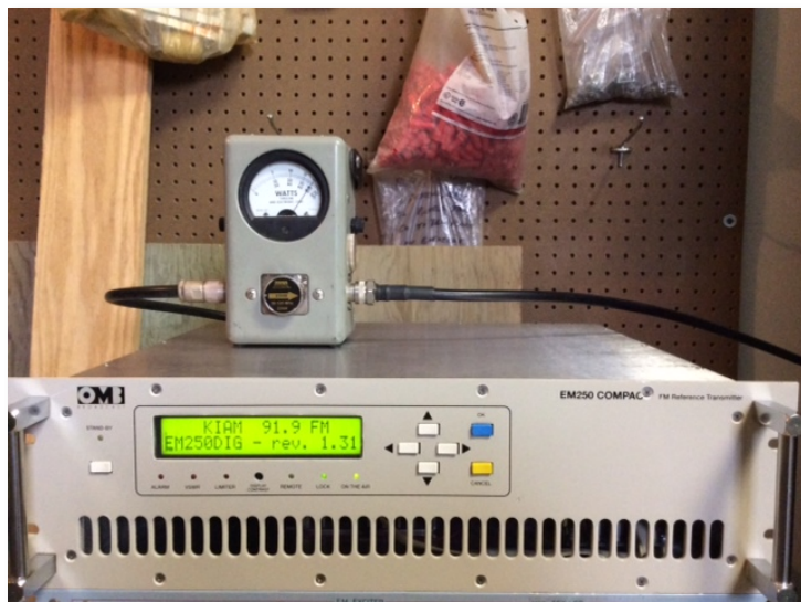
Modern solid-state FM transmitter
